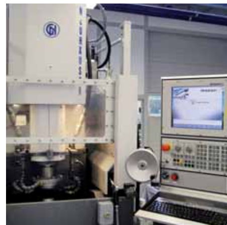
↑ Surface grinder for flat and hollow grinding of disk-shaped cutting tools
